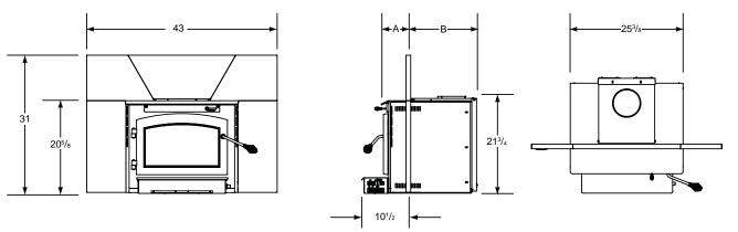
\* A and B are adjustable in 3/8" increments (see min max below).
