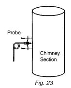
For the probe (fig. 23), drill a hole in the side of the chimney, attach the mounting plate over it with the
