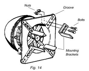
Adjust the final position of the installation brackets ensuring that there is clearance between the brackets and the flue wall.
