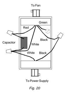
The diagram below shows the connections for the entire system.
