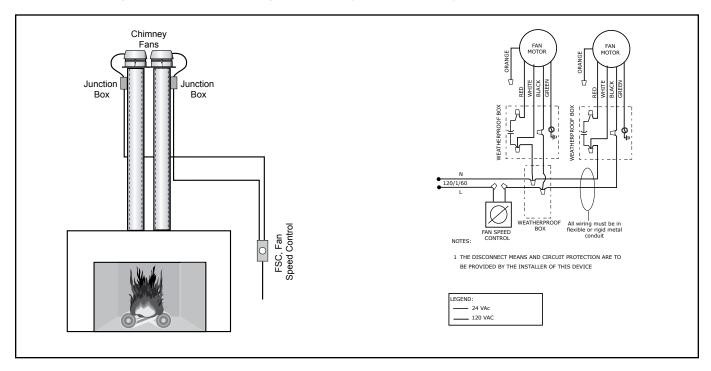
The diagrams below show the wiring of two chimney fans and how they are connected to the fan speed control.
